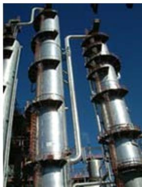
■ Distillation method: Method of conducting vacuum distillation using a distillation tower with a height of 30 meters or more to separate light water and heavy water (multiple distillation processes are necessary)
